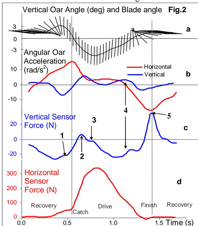
As the oar squared and feathered during the stroke cycle, the orientation of the sensors is changing relative to the horizon. Therefore, the oar roll was measured with **BioRow** 7D sensor (RBN 2012/10), so the orientation of the blade and sensors was determined (Fig.2, a). Angular oar accelerations (Fig.2, b) were
