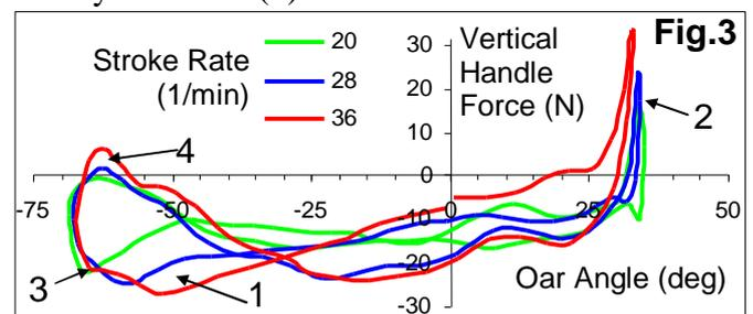
Concluding, vertical forces at the handle are quite small and even smaller at the blade (about 10N ~ 1kgF), so they do not really contribute to vertical movements of the rower-boat system.
